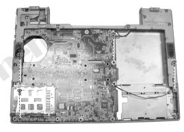
Figure 2-27 Disconnect the cables and separate the rear covers
